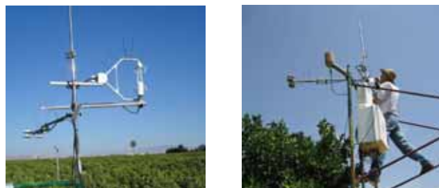
Figure 15 shows the installation process of the measuring equipment used by the Universidad Politécnica de Cartagena.
